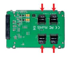
Insert 2 or 4 MicroSD cards into the MicroSD card slot.
