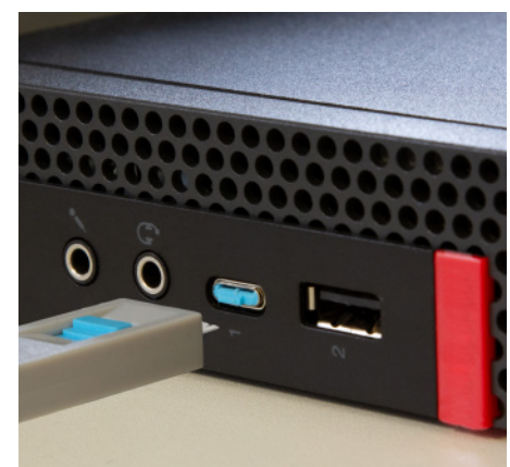
Push the button backwards and pull out the Key. The USB-C port is locked.
