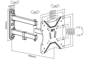
Install the wall plate to the wall
